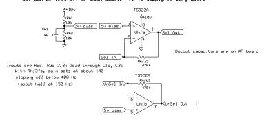
This circuit is built on a plug in card that sockets instead of an LA4525
